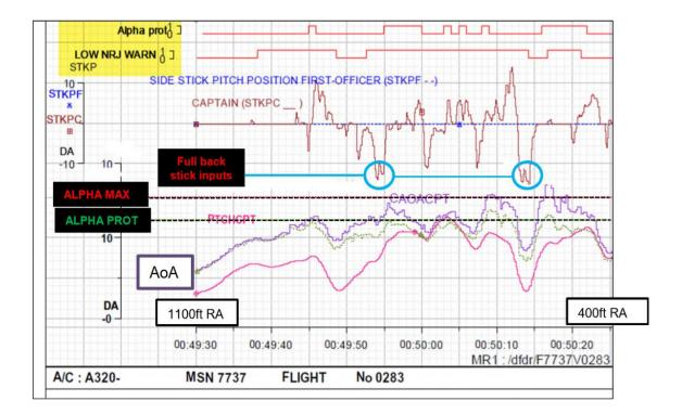
PF carried out manual approach. Between 1000 ft to 400 ft RA, high activity was recorded on Pilot Flying side stick. Pitch varied between 3° and 12° nose up and Roll varied between 0° and 10° (right wing down). Vertical descent rate varied between 0 ft/ min and 1600 ft/ min. CAS varied between 125 kts and 113 kts (VLS was 127 kts).
